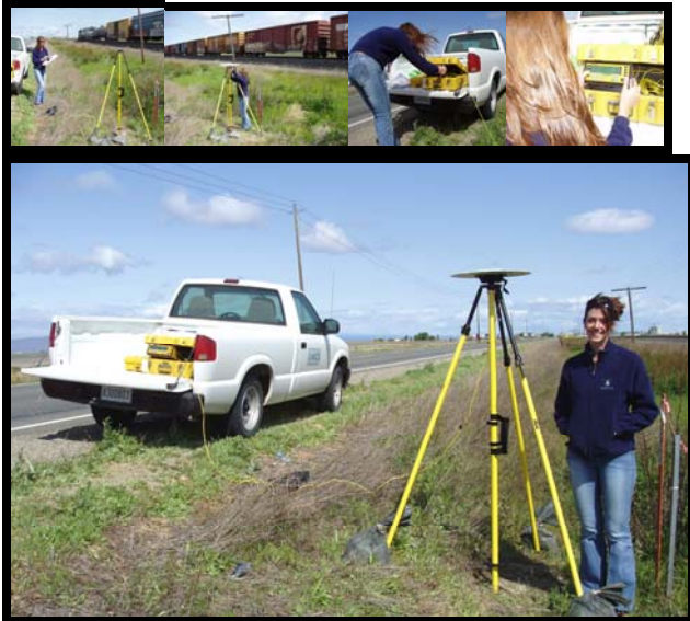
Above: WC sets up subsidence monitoring equipment (Old Hwy 99W - North of Arbuckle) to facilitate information gathering for the Sacramento Valley Height Modernization Project. Information collected through this collaborative process will help direct future groundwater planning and management within the watershed.
